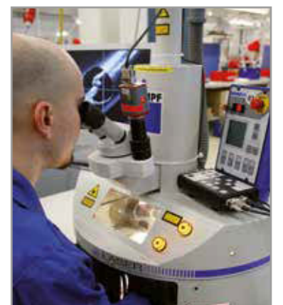
The very latest production techniques are used the sensor manufacturing, for eg. laser welding machines.
