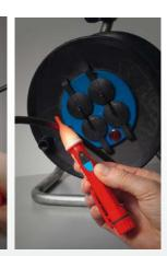
Testing of cable breaks
