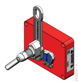
The SOL latch lock is a key access interlock is suitable for use on hinged and sliding doors. The interlock is manufactured in copper brushed aluminium, making it ideal for use in harsh or corrosive environments and heavy use. Typical industries using the SOL latch lock are chemical, aggregate & concrete, iron & steel, paper & wood transformation, rail and power generation.
