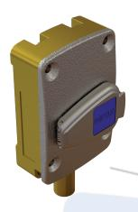
The MS bolt lock is a mechanical lock with a trapped key, suitable for electrical locking (disconnecting switch, circuit breaker, etc.). This model of MS allows the rotation of the power switch gyratory or the movement of the shaft of a disconnector lever to be controlled.
