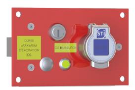
the ERTK is an electromechanical key switch. The release (SP) or trapping (RP) of the key are electrically controlled. Any change in the key status is signalled by the switch connected to the lock. The ERTK is particularly suitable for automated systems in industry or railway equipment.
